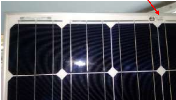
RFID Tag position outside the laminate
